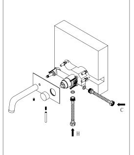
Please check that your pressure is suitable for this product before installation, details can be found on our website, recommed minimum working pressure: 0.5 bar, maximum working pressure: 3 bar
